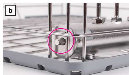
Control indicator has triggered
